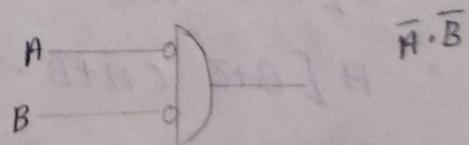
NAND gate is equivalent to bubbled OR gate:-
