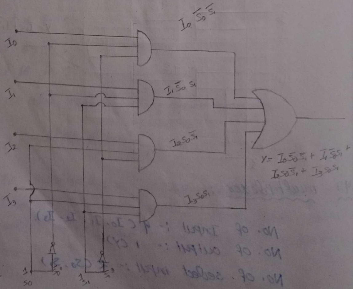
$$Y = I_0 \bar{S}_0 \bar{S}_1 + I_1 \bar{S}_0 S_1 + I_2 S_0 \bar{S}_1 + I_3 S_0 S_1$$
